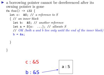
▶ a borrowing pointer cannot be dereferenced after its owning pointer is gone fn foo() -> i32 { let c: &S; // a reference to S { // an inner block let b: &S; // another reference let a = S{x: ...}; // allocate S // OK (both a and b live only until the end of the inner block) b = &a;c = b; // dangerous (c outlives a) c : &S
